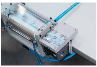
Fig.: Automatic Pull Through Device of ROLL2BASKET
