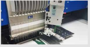
Fig.: Cording Device EP 1.2 at ZSK F-Head
