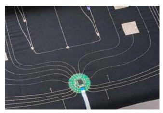
Electronic board placed on fabric and connected with conductive threads.
