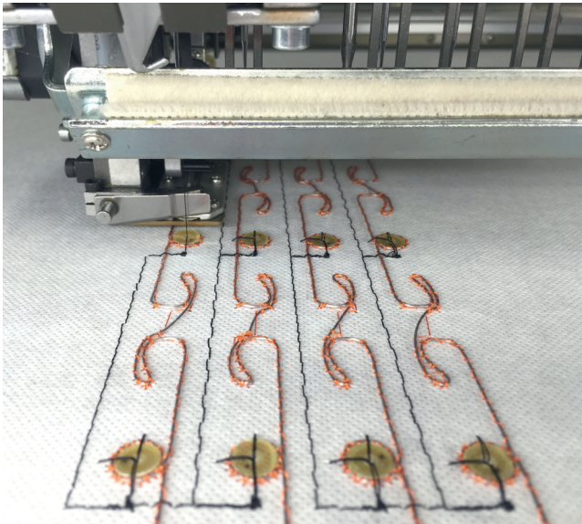
RFID antennas placed and fixed by embroidery.
