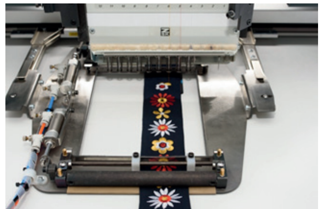
Fig.: Automatic Clamping Frame of ROLL2BASKET
